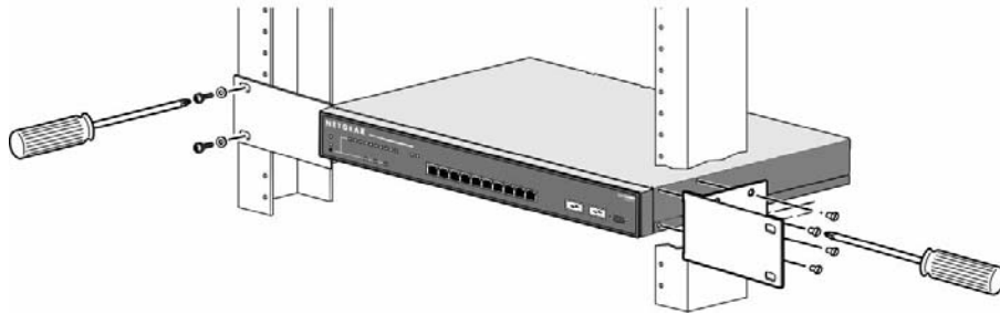
Figure 3-1. Attaching Mounting Brackets
